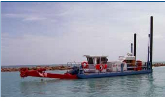
370-20 (6 m) dredging a marina
