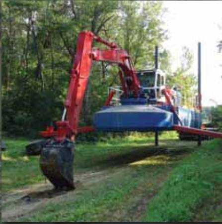
Mobilizes Without Crane, Self Launches
